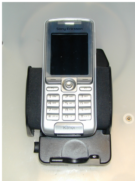
Fig. 1 Position of the phone in to the Rohde&Schwarz holder.
